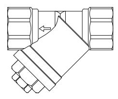
PRODUCT DESCRIPTION: The USIS Model YS is a female NPT brass wye strainer that is designed to protect piping systems from damage cause by dirt and debris. The YS comes standard with a 20-mesh filtering screen, a  $\frac{1}{4}$ " tap for blow out on sizes  $\frac{1}{2}$ " - 1- $\frac{1}{4}$ ", and a  $\frac{1}{4}$ " tap for bow out in the 1- $\frac{1}{2}$ " and 2" sizes.
