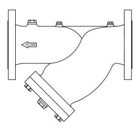
PRODUCT DESCRIPTION: The USIS CYS is a flange x flange end wye strainer. The cast iron wye strainer has standard ANSI Class 150 pound flange ends. The wye strainer comes standard with a stainless steel filter element, two  $\frac{1}{2}$ " plugs, a  $\frac{1}{2}$ " plug, a plugged  $\frac{3}{4}$ " blow-off connection, and a flanged blow-off cover with an EPDM o-ring.
