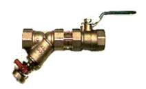
Product Description: Ball valve, wye-strainer are rated at 600 WOG. CBY uses a full port ball valve connected to the strainer with a standard hose nipple. The strainer has a ¼" tap in the blow down section for a drain with a 20 mesh stainless steel screen. All taps are pluged unless options are specified. The CBY assembly is pressure tested under 100 PSI air to ensure no leakage. Connections include sweat or female on the ball valve side and female on the strainer side.
