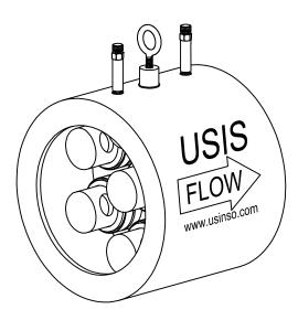
PRODUCT DESCRIPTION: The USIS AFLW is a wafer type Automatic Flow Limiting Device with a full flange face. The AFLW is designed to fit between two ANSI Class 150 pound flanges. The AFLW is supplied with one or more stainless steel flow limiting cartridges that can be removed for cleaning, inspection, and, if necessary, cartridge exchange. The AFLW has two predrilled openings for pressure/ temperature ports, a drain plug, and a lifting lug for ease in installation.
