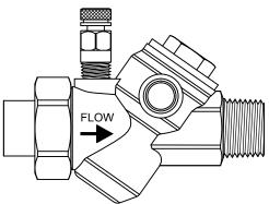
PRODUCT DESCRIPTION: The USIS AFLD is an Automatic Flow Limiting Device, male ended by union, rated at 600 WOG. The AFLD is supplied with a stainless steel flow limiting cartridge that can be removed for cleaning, inspection, and, if necessary, cartridge exchange. The AFLD comes standard with two pressure/temperature ports and a hanging ID tag for easy identification. The union side connections are available in NPTM, NPTF, SWT, and a variety of reductions.
